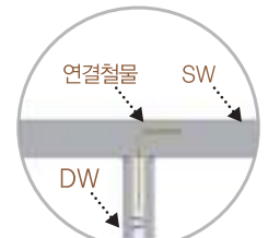
D. SW-DW Joint #2.
